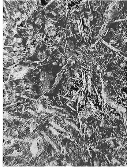
Figure 1: Basalt with an intersertal texture, Hole CY-1, 348.1 m, magnification \times 150 .
