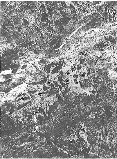
Figure 7: Crystalline fragments in altered glass, glassy breccia, Hole CY-1A, 455.2 m, magnification \times 150 .
